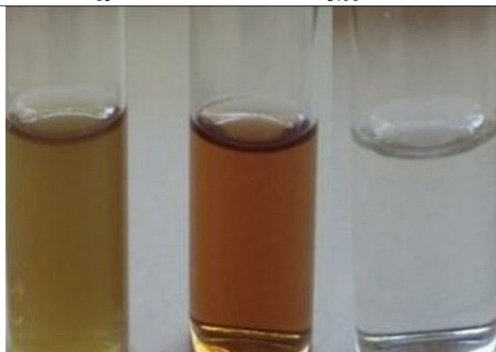
Figure 1: Colour Change of synthesized TiO 2 nanoparticles from ethanol extract of Citrus reticulata peels
